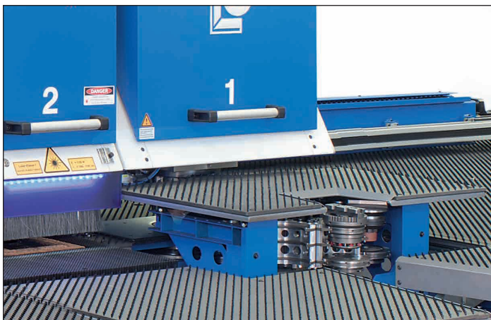
CombiLaser Multipunch with automatic tool changer
