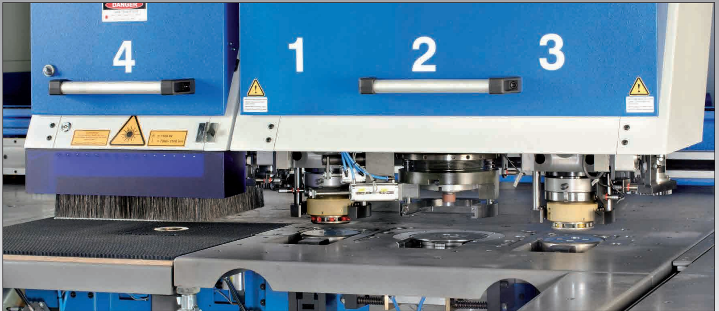
CombiLaser TRI 3-head punching machine with 2xRevotool (head 1 + 3) and rotation / index (head 2)
